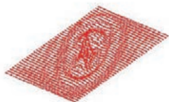
Fig. : Crinkling at a Stone-Wales defect
